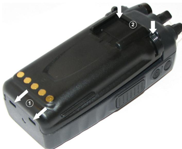
Figure 3-1: Attaching the Battery
