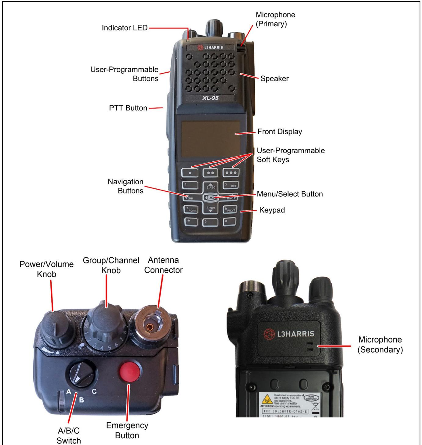
Figure 4-1: Radio Controls, Indicators, and Connectors
