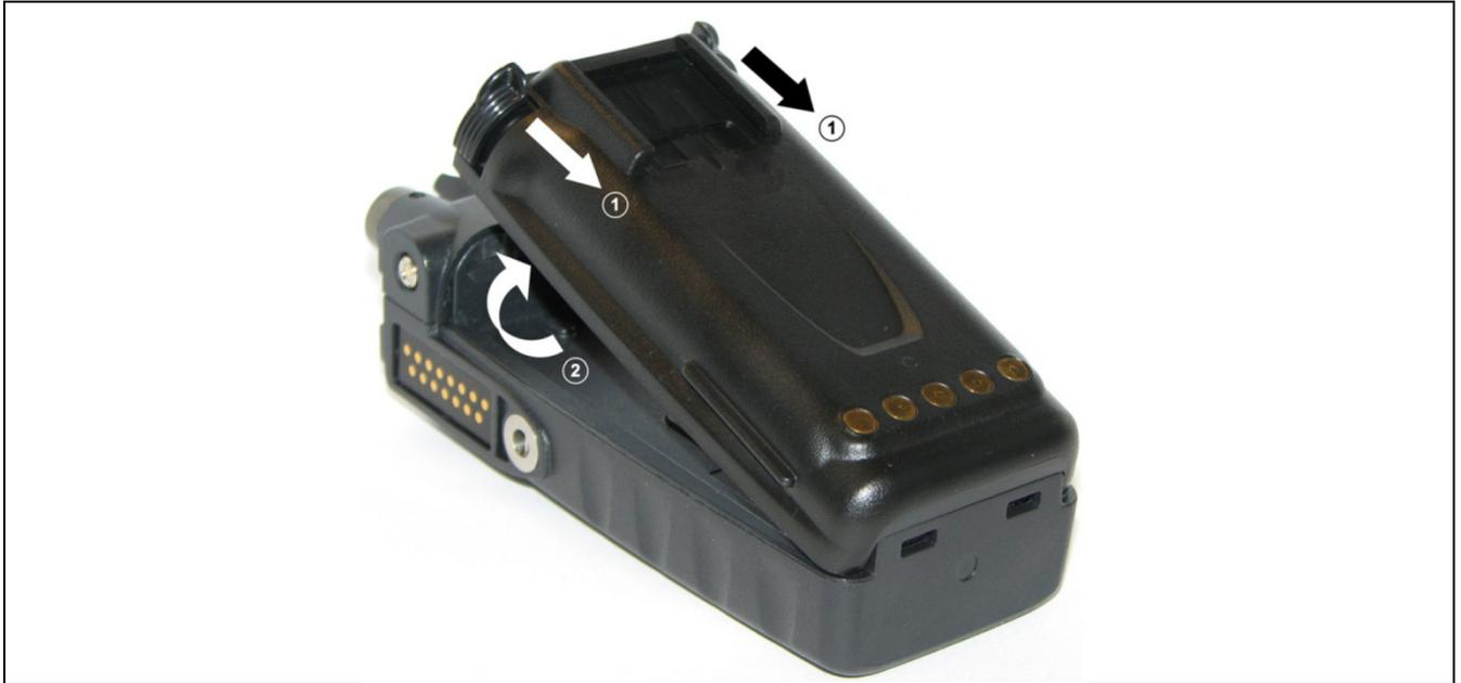
Figure 3-2: Remove the Battery
