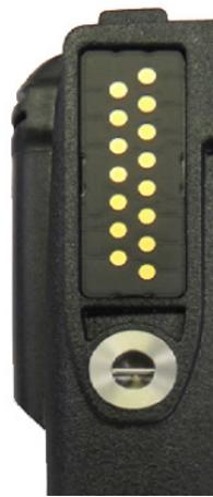
Figure 3-3: Universal Device Connector
