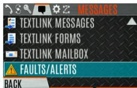
4. Fault messages are displayed. Press the up or down navigation buttons to highlight the desired fault. Press the **OPTIONS** soft key delete faults. Press the **DETAILS** soft key to view details for the highlighted fault.
