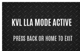
4. Once KVL LLA Mode is activated, the KVL-5000 can be used to provision the radio with LLA keys. The radio will remain in KVL LLA Mode until the user exits this state.
