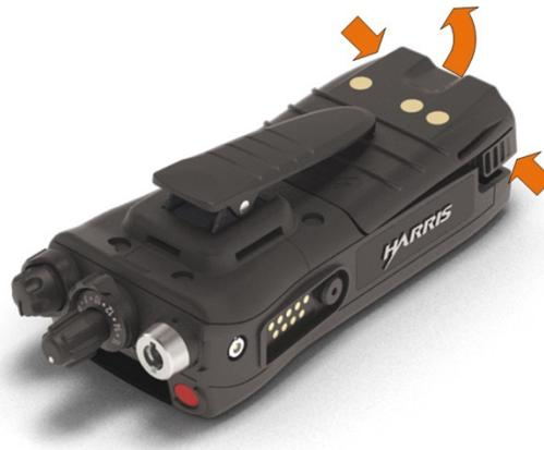
Figure 4-2: Remove the Battery
