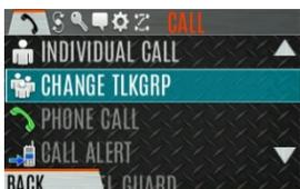
4. Press the up or down navigation buttons to highlight and the desired talkgroup and press the Menu/Select button. After selecting the new talkgroup, the radio returns to the main screen.
