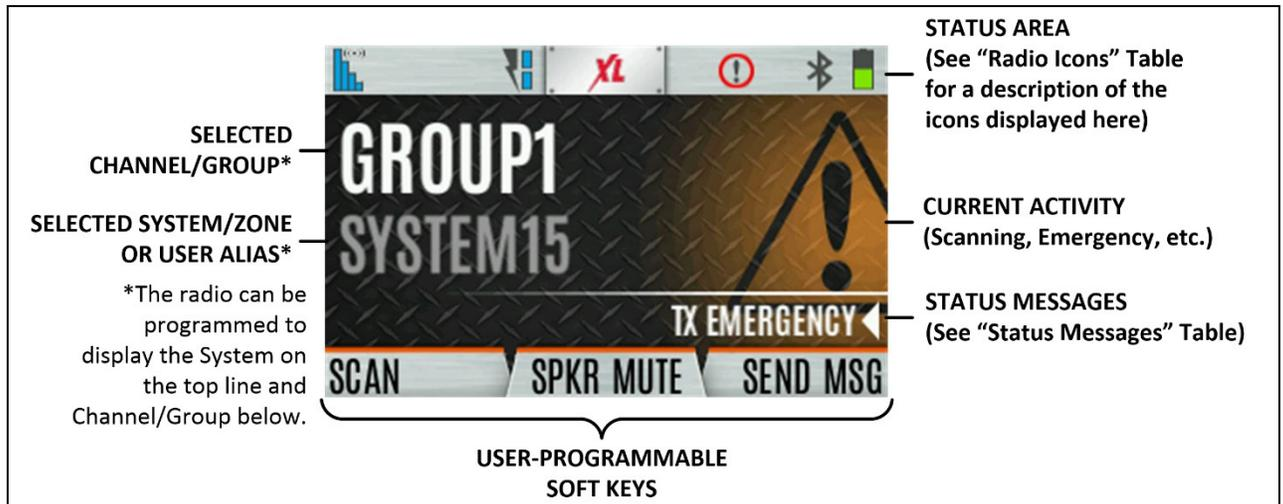
Figure 5-4: Sample Idle Front Display
