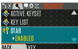
4. Press the up or down navigation buttons to select **OTAR REKEY** and press the Menu/Select button to request that the KMF updates the keys in the radio. **OTAR REKEY** is only enabled if the radio has successfully registered for data operations. If enabled via programming, the radio plays an audible confirmation tone to indicate successful OTAR rekey.
