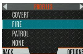
5. Press the up or down navigation buttons to select the desired Profile and press the Menu/Select button.
