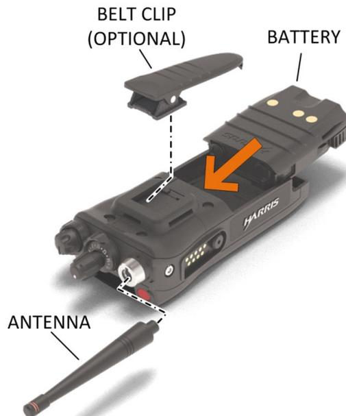
Figure 4-1: Radio Assembly
