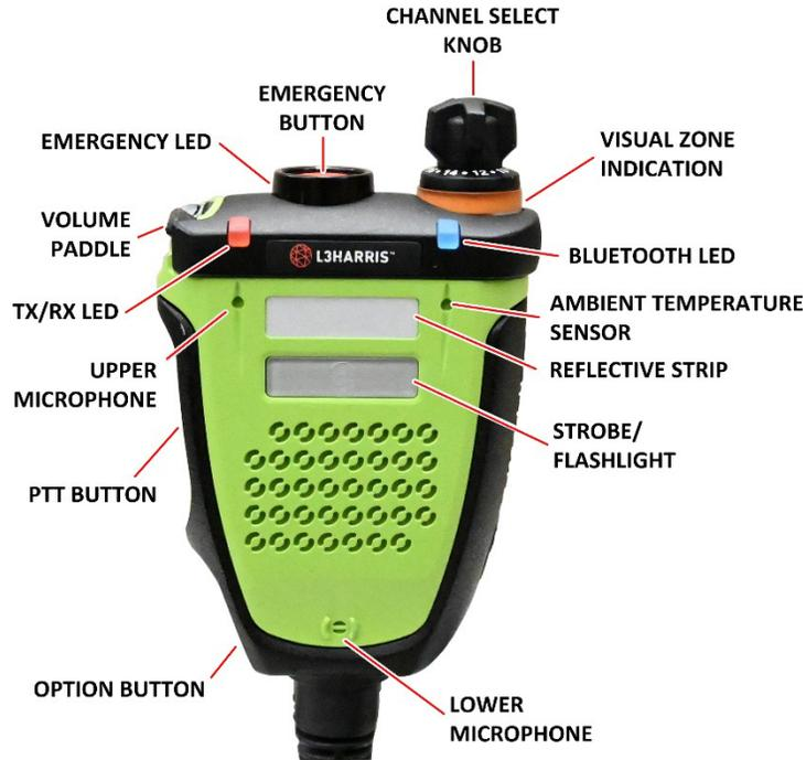
**Figure 5-2: XL Extreme Speaker Microphone Controls**
