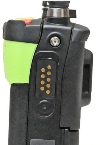
Figure 4-3: Universal Device Connector
