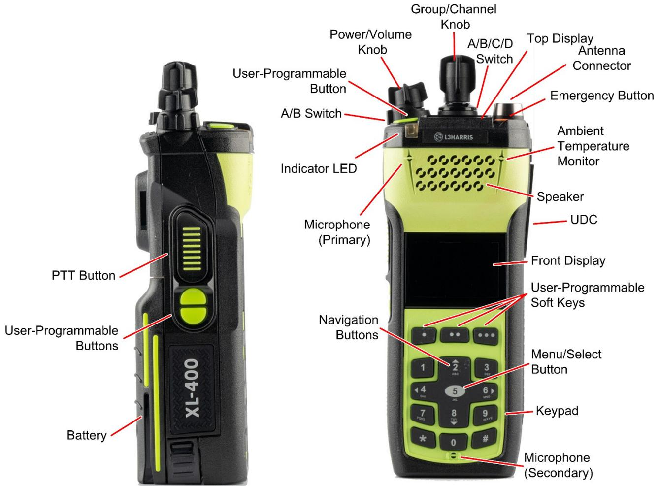
Figure 5-1: Radio Controls
