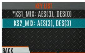
5. Select the desired keyset and press the Menu/Select button to display the individual keys. Highlight the desired key and press the **Delete** softkey.
