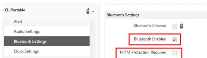
8. Program a radio button or switch for Bluetooth Enable/Disable:
