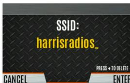
5. Highlight and select PASSWORD. Use the keypad on the radio to enter the password.
