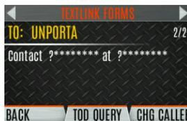
5. Enter text into blank field(s) (up to eight alphanumeric characters) and press the **NEXT** soft key.
