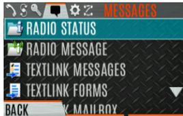
4. Use the up or down navigation buttons and the Menu/Select button to highlight and select desired status.
