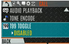
4. Press the Menu/Select button to change **T99 TOGGLE** between **ENABLED** and **DISABLED**. **T99** is displayed in the top of the radio display when Type 99 is enabled.
