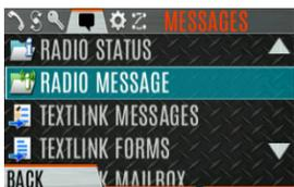
4. Use the up or down navigation buttons and the Menu/Select button to highlight and select the desired message.
