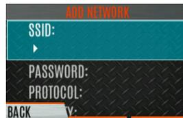
4. Highlight and select SSID. Use the keypad on the radio to enter the SSID and press the **ENTER** softkey.
