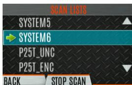
5. Press the up or down navigation buttons to highlight the desired channel.
