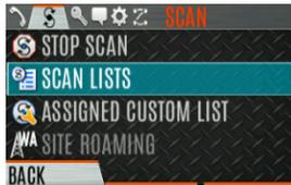
4. Press the up or down navigation buttons to highlight the scan list and press the Menu/Select button. When scanning is started, ➔ indicates the active scan list; when scanning is stopped, 📶 indicates the active scan list.
