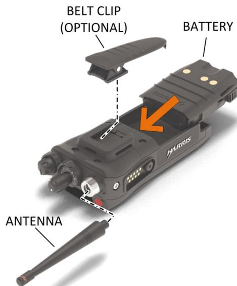
**Figure 4-1: Radio Assembly**
