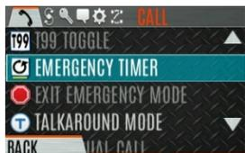
4. Set the Emergency Check-In Timer using the left or right navigation buttons. The minimum and maximum allowable values are programmed via RPM2. Default is 10 minutes.
