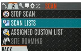
4. Press the up or down navigation buttons to highlight the scan list and press the Menu/Select button.
