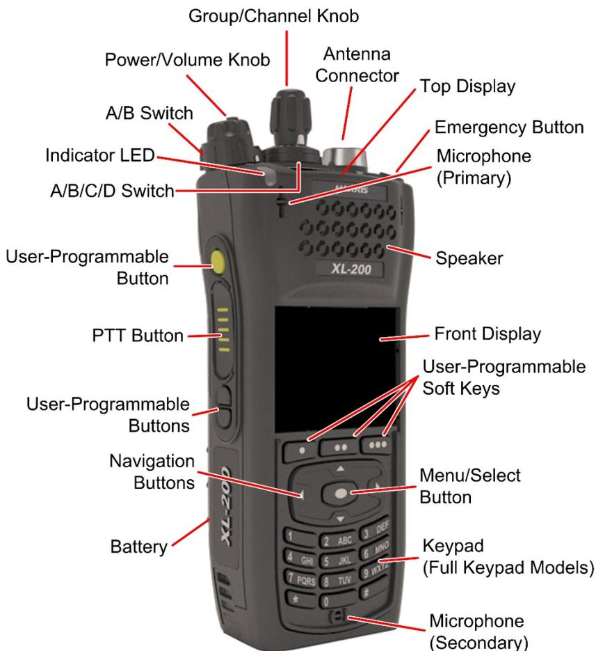
**Figure 5-1: Radio Controls**
