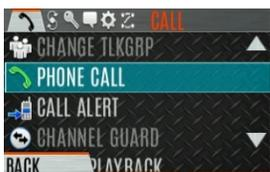
4. Select an entry from the list of pre-programmed entries or click **DIRECT DIAL** to enter the number directly. Direct Dial entries can have up to 31 characters (0-9, \*, #, or a space; the space correlates to a pause.) Select **OPTIONS** to view details about the highlighted pre-programmed entry. The radio supports up to 255 pre-programmed entries.
