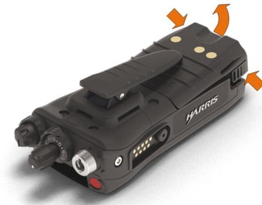
Figure 4-2: Remove the Battery
