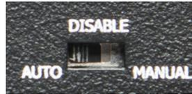
Figure 6-12: Backup Radio Switch
