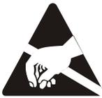
The solid-state drive is susceptible to the effects of **Electro-Static Discharge (ESD)**. When handling the solid-state drive, use a grounded wrist strap to prevent ESD from damaging the solid-state drive.
